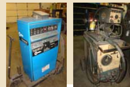
LEFT PIC: MILLER SYNCROWAVE 351 TIG WELDER
