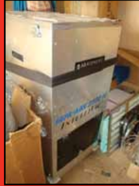
COMPLETE ABATEMENT DUCT CLEANING SYSTEM
