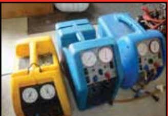
VAPOER & LIQUID RECOVERY SYSTEMS
