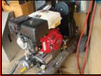
GAS POWERED ABATEMENT COMPRESSOR...PART OF DUCT CLEANING SYSTEM
