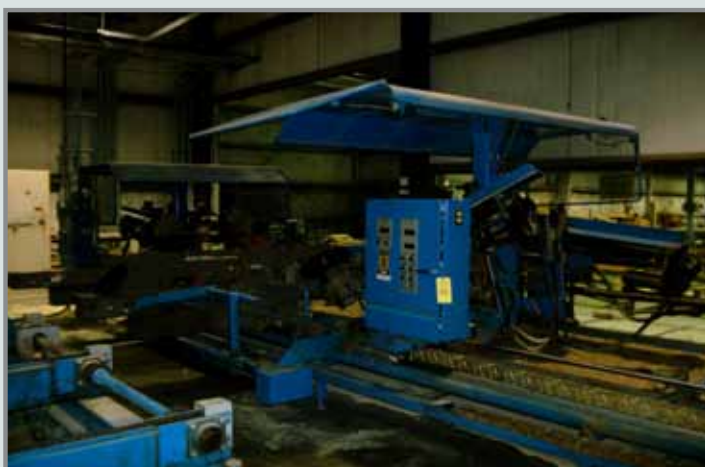
1998 KOSKOVICH AUTO OMNI COMPONENT SAW 5 BLADE COMPUTERIZED SAW; (3) APEX DIGITAL INCLINOMETERS & SELF CLEANING MAIN DRIVE NUT; ALL FACTORY OPTIONS INCLUDING REMOTE SIDE MONITOR & MATTHEWS INK JET PRINTER; SHAKER PAN CONVEYOR
