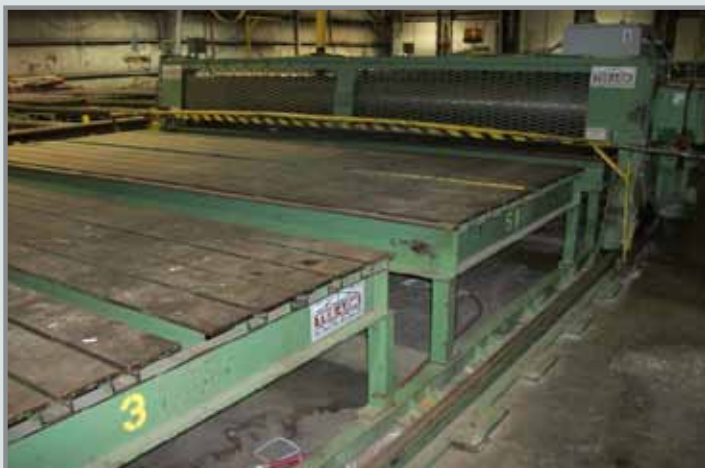
1999 TEE-LOK SIDE EJECT 24" DIAMETER GANTRY 96' SIDE EJECT SYSTEM WITH (13) TEE-SLOT 6'X14' TABLES WITH RECESSED TAPE MEASURES, (2) TEE-LOK 14'X24" DIAMETER ROLLER GANTRIES, SOFT START DIRECT DRIVE GEAR MOTOS. SYSTEM INCLUDES MANIFOLD AND AVAILABLE JIGGING HARDWARE
