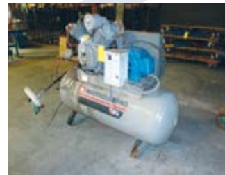
INGERSOLL RAND T30 AIR COMPRESSOR
