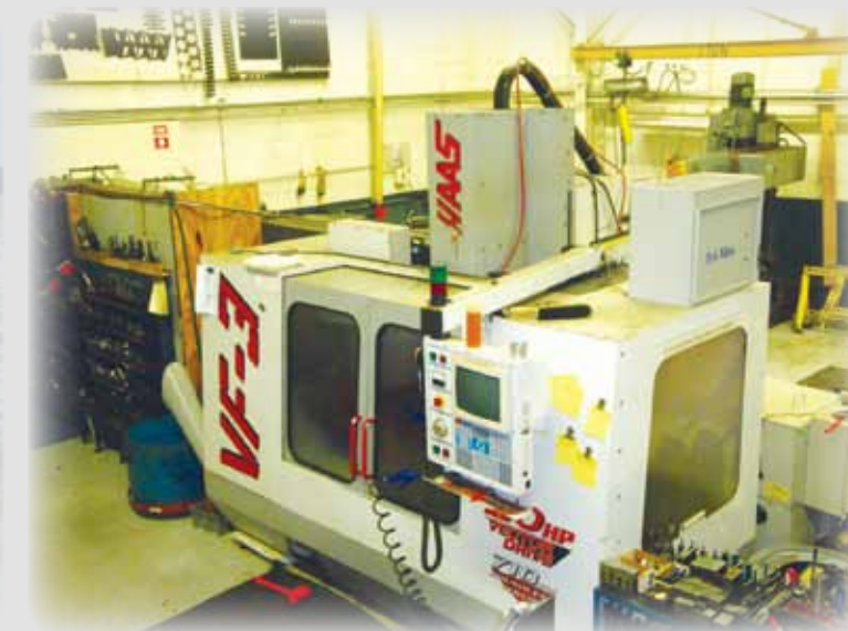
1998 HAAS VF-3 VERTICAL MACHINING CENTER
