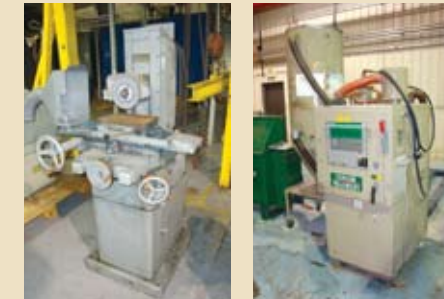
LEFT PIC: (6X18) HANDFEED SURFACE GRINDER RIGHT PIC: CONAIR FRANKLIN VACUUM LOADER
