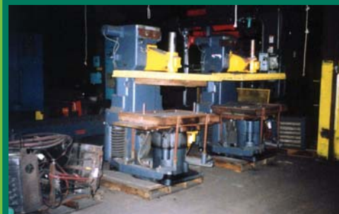
(2) BMM CT-3 MOLDING MACHINES
