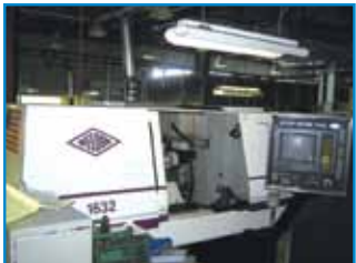
WELDON ID/OD CNC Hydraulic Grinder with GE Fanuc series 150-t CNC Controller. Model #1632, Serial # 761.
