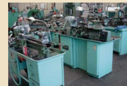
(OVER 5) HARDINGE & SOUTH BEND SECOND OPERATION LATHES
