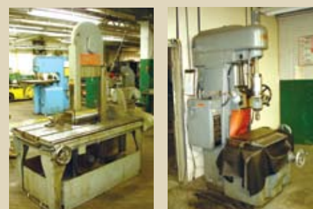
LEFT PIC: MARVEL VERTICAL BAND SAW RIGHT PIC: MOORE JIG BORER, NO.3
