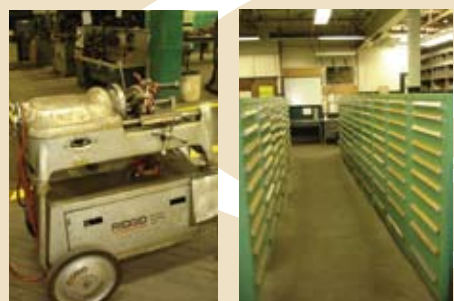
LEFT PIC: RIDGID 535 POWER THREADER RIGHT PIC: (OVER 50) VIDMAR CABINETS
