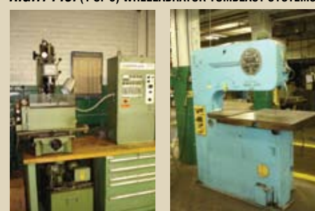
LEFT PIC: CHARMILLES D-10 SINKER EDM RIGHT PIC: DO ALL 36" VERTICAL BAND SAW
