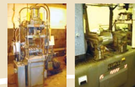
LEFT PIC: (1 OF 30) STOKES COMPRESSION MOLDING MACHINES RIGHT PIC: EEMCO LAB MILL
