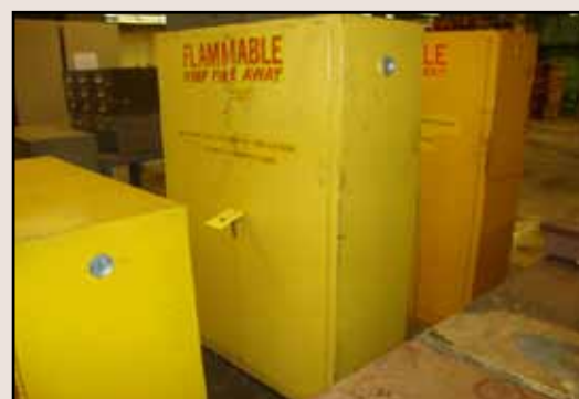
FLAMMABLE STORAGE CABINETS
