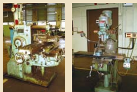
LEFT PIC: 1 OF 2 MILWAUKEE MILLING MACHINES RIGHT PIC: BRIDGEPORT VERTICAL MILL 2 HP
