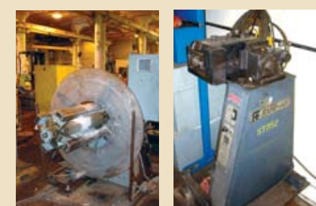
LEFT PIC: LITTELL CENTERING REEL RIGHT PIC: RAPID AIR STOCK FEEDER
