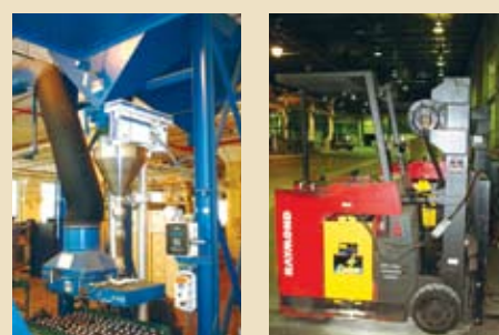
LEFT PIC: LIQUID CORP SAND PACKING MACHINE RIGHT PIC: RAYMOND ELECTRIC FORKTRUCK
