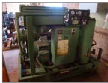
SULLAIR ROTARY SCREW AIR COMPRESSOR
