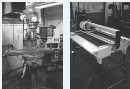
LEFT: (1 OF 2) BRIDGEPORT VERTICAL MILLS RIGHT: 2007 QEP TILE SEW
