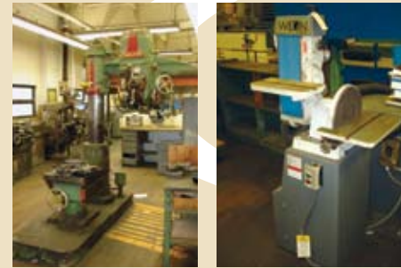
LEFT PIC: CARLTON RADIAL ARM DRILL RIGHT PIC: WILTON DISC & BELT SANDER
