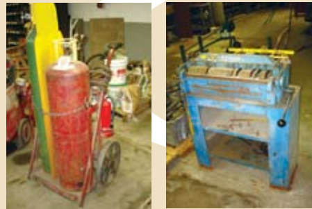
LEFT PIC: OXYGEN AND ACETYLENE TORCH SET RIGHT PIC: PEXTO FINGER BRAKE
