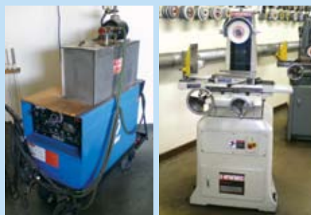
LEFT PIC: MILLER Dialarc HF Welding Unit RIGHT PIC: HARIG Surface Grinder
