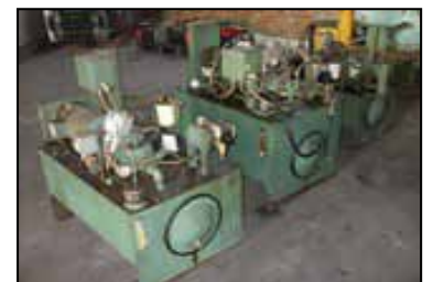
OIL CIRCULATING TANKS
