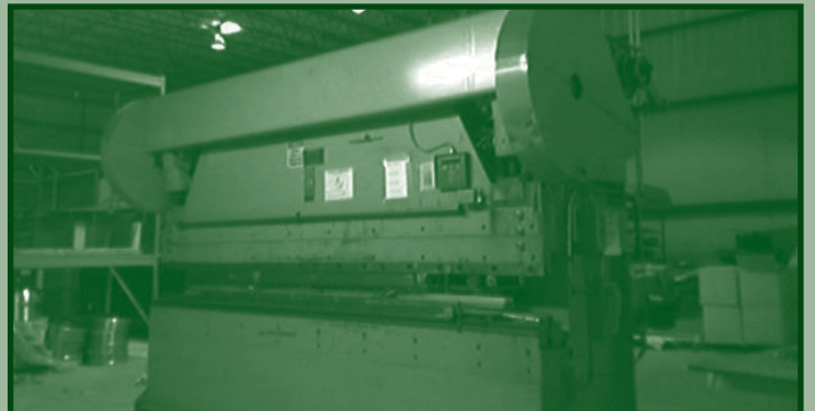
BATH 10' X 1/4" HYDRAULIC BRAKE PRESS
